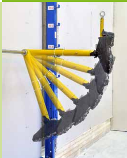
Figur 2: Hard Body Impact, Gyproc modifisert, ISO 7892 part 2 1998 30 N m
