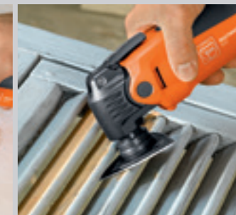
Flat slipeplate for smale mellomrom.
